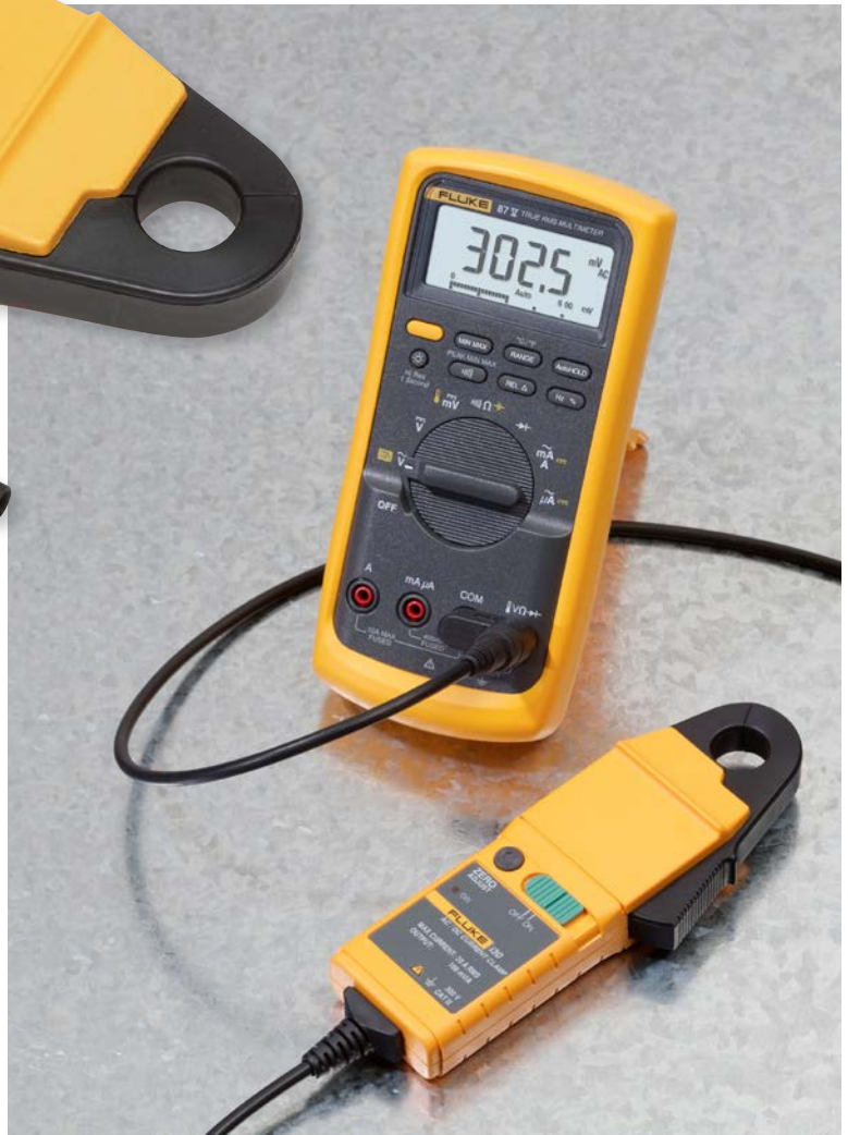
i30 connected to a Fluke 87V Digital Multimeter
